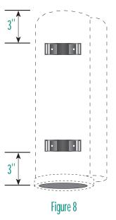
3. Place each mounting base under the Bazooka so that the apex at the bottom of the tube sits inside the mounting base as in figure 7.
